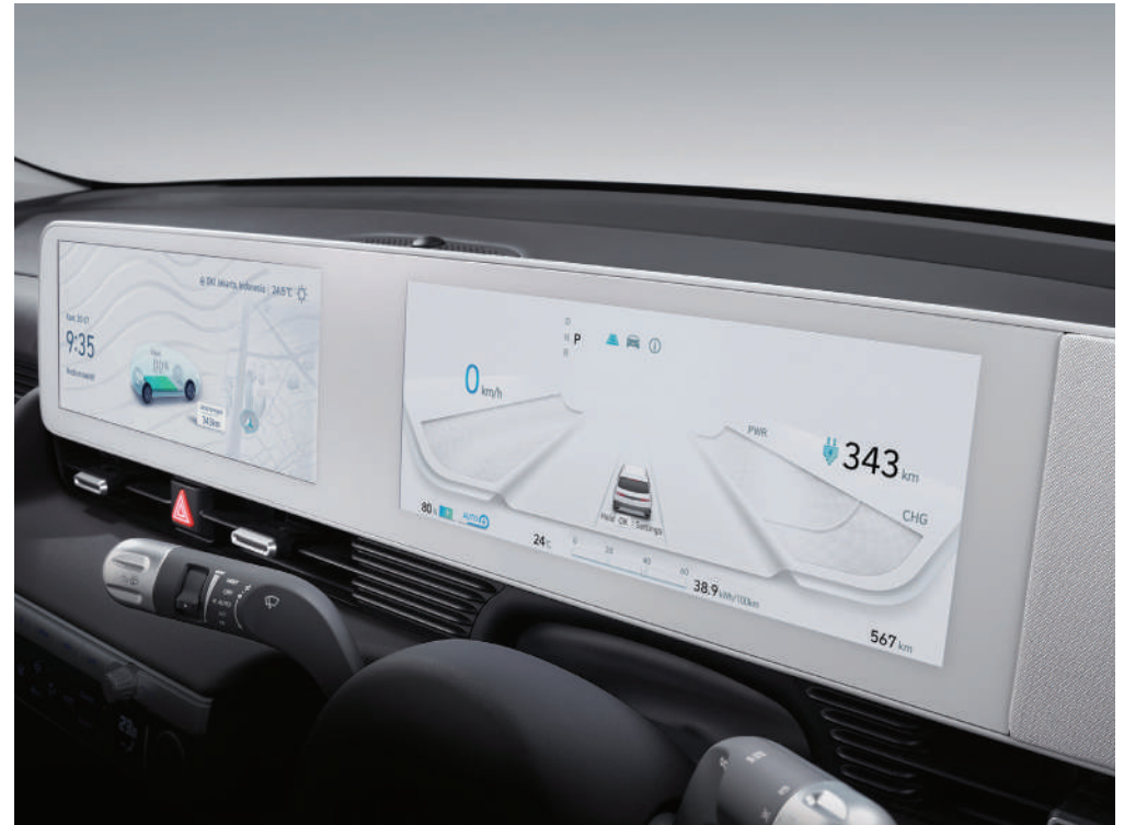
12.3" TFT LCD Cluster with integrated A/V System
