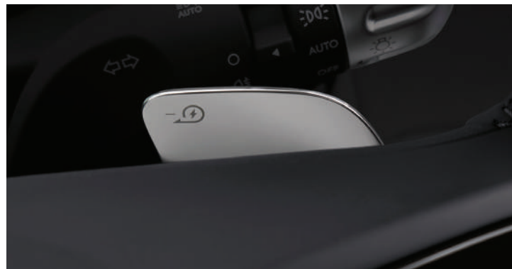
Paddle Shifter for Regenerative Braking
